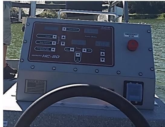
*Our new control box capable of generating 80 amps. Although not perfect for conductivities great than 2,500 microsiemens, it should definitely be an improvement.*
