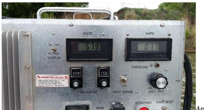
*Example of the older style of electrofishing control box capable of generating 40 amps. While great in typical systems, this unit struggles in high conductivity systems.*
