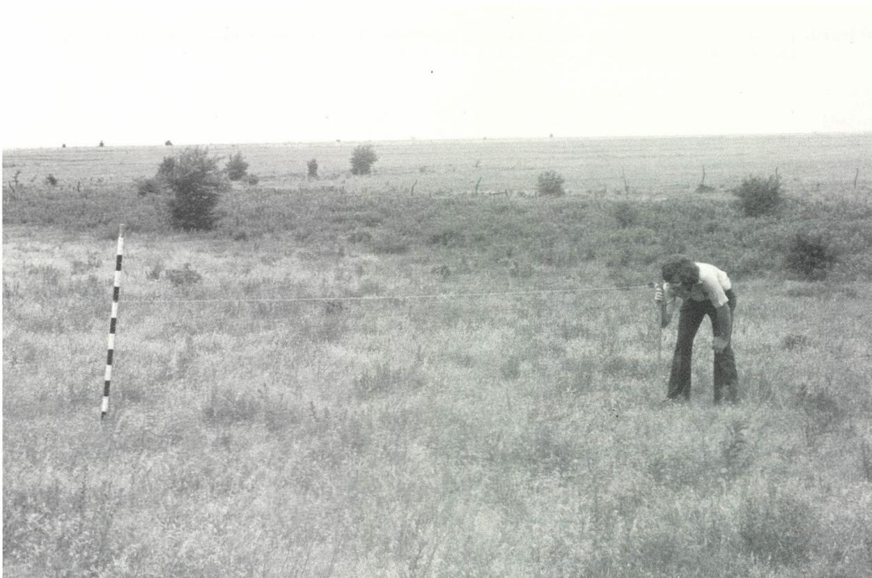
Figure 16. A modified vegetative step point measuring device used to determine vegetative composition and basal cover at prairie chicken activity areas and along transects on the grassland-cropland study area in Chase County, Kansas, 1975-1978.
