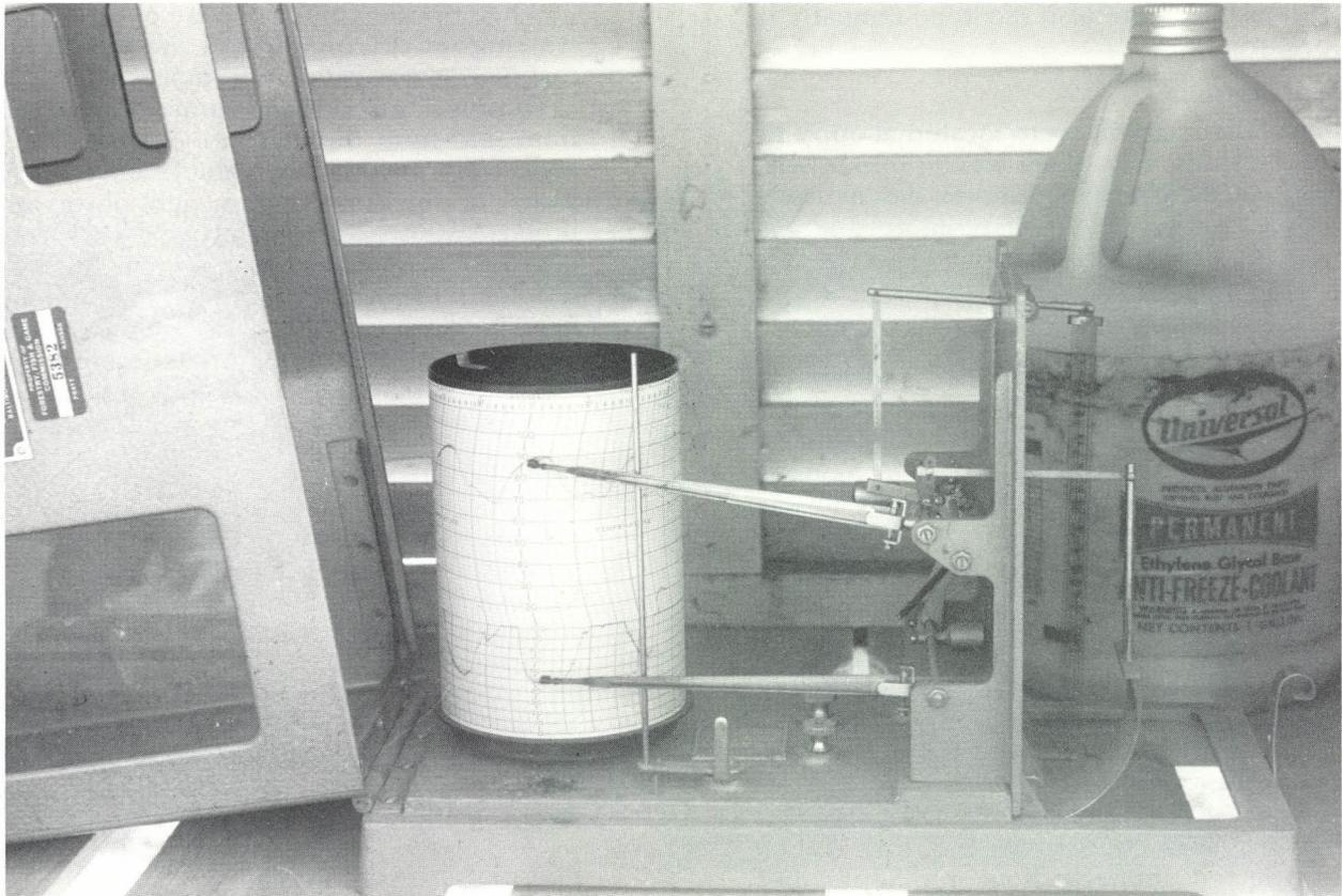
Hydrothermograph for a 7 day constant recording of temperature and humidity.
