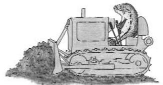
installed. Dams pushed up with a dozer and not compacted have a greater chance of failure.
